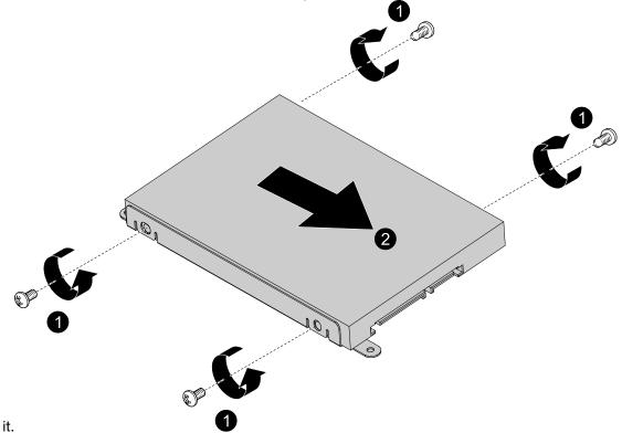
Step 9. To install the new hard disk drive as follows:
