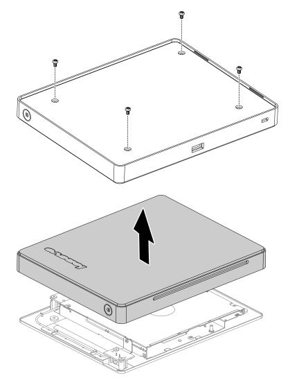
Step 5. Remove the 3 screws and slide the optical disk drive out as shown.
