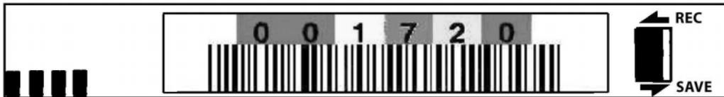
**Figure 4-4** Example of a bar code label attached to a data cartridge.
