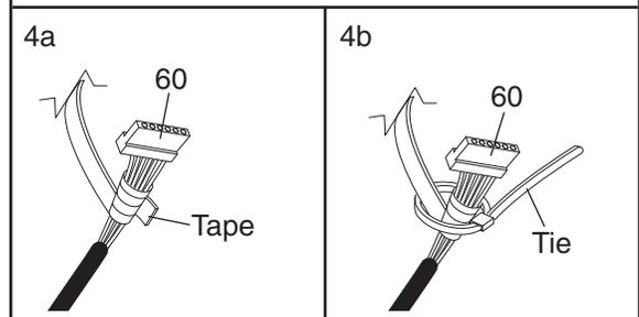
5. Carefully pull the opposite end of the tape to pull the Wire Harness (60) up through the Right Handrail (59) and out of the hole in the side of the Right Handrail.
