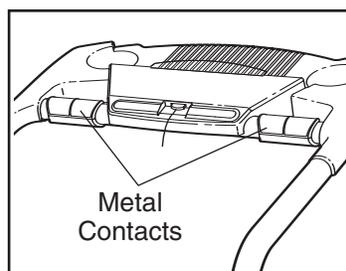
To measure your heart rate, **stand on the foot rails** and hold the metal contacts on the pulse handgrips—**avoid moving your hands**. When your pulse is detected, the heart symbol in the Pulse zone of the display will begin to flash each
