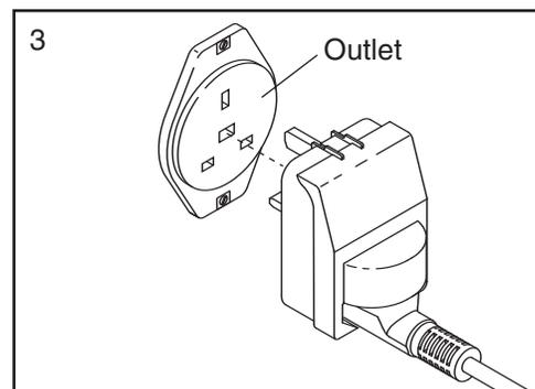
**⚠ DANGER:** Improper connection of the equipment-earthing conductor can result in an increased risk of electric shock. Check with a qualified electrician or serviceman if you are in doubt as to whether the product is properly earthed. Do not modify the plug provided with the product—if it will not fit the outlet, have a proper outlet installed by a qualified electrician.
