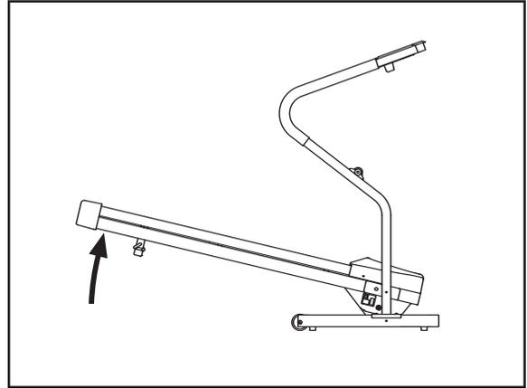
2. Move your right hand to the position shown and hold the treadmill firmly. Using your left hand, pull the lock knob to the left and hold it. Raise the frame until it passes the lock pin. Slowly release the lock knob. **Make sure that the frame is securely held by the lock pin.**
