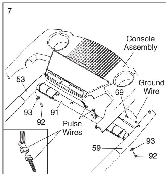
With the help of a second person, hold the console assembly near the Crossbar (91). Connect the pulse wire from the Crossbar to the pulse wire from the console assembly. **The connectors should slide easily into each other and snap into place.** If they do not slide easily and snap into place, turn a connector and then insert it.
