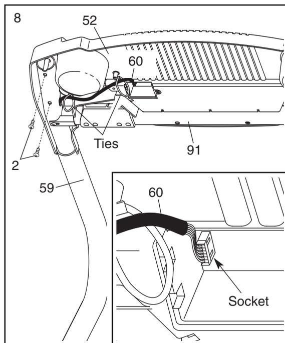
Insert the Wire Harness (60) through the two indicated plastic ties on the Console Base (52). Next, **touch the Right Handrail (59) to discharge any static.** See the inset drawing. Insert the connector on the end of the Wire Harness into the red socket beneath the console. **The connector should slide easily into the socket and snap into place.** If the connector does not slide easily and snap into place, turn the connector and then insert it.
