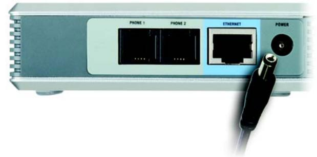
**Figure 3-4: Connect the Power**
