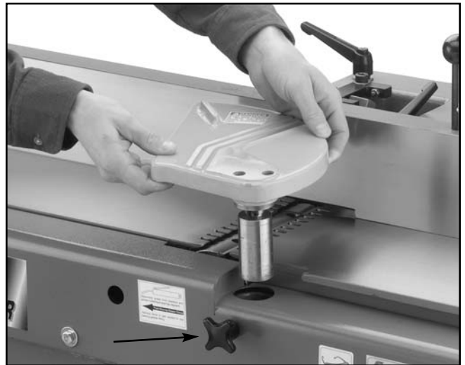
Figure 6a. Attaching cutterhead guard.
