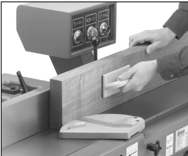
Figure 19. Operator position for edge jointing.
