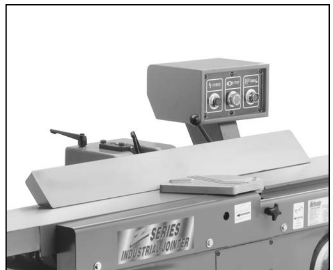
Figure 20. Fence position for bevel jointing.
