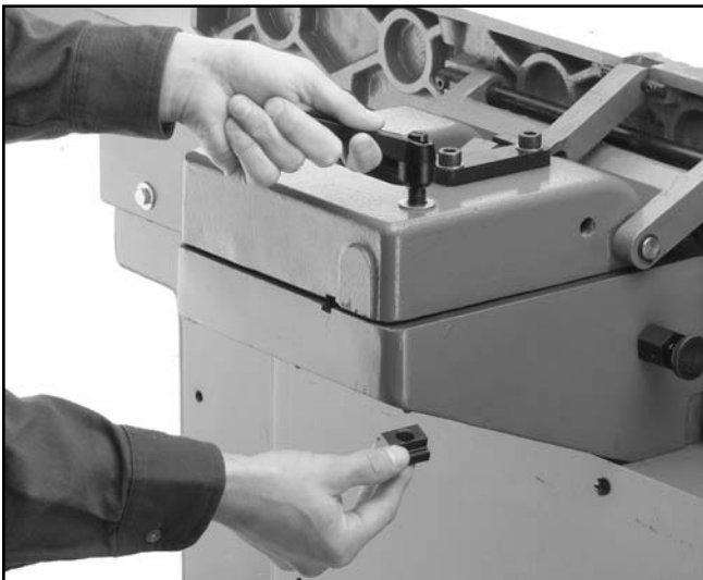
Figure 5. Fence base lock knob attachment.
