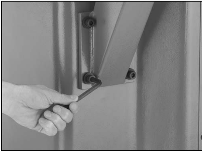
Figure 7A. Mounting the pedestal switch.
