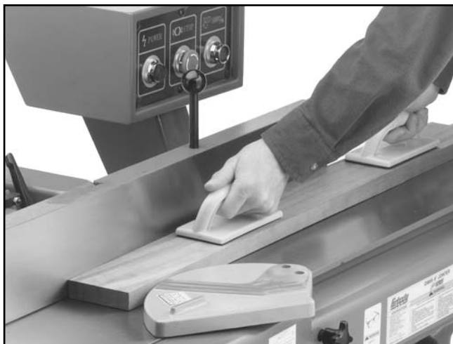
Figure 21. Correct method for surface planing.
