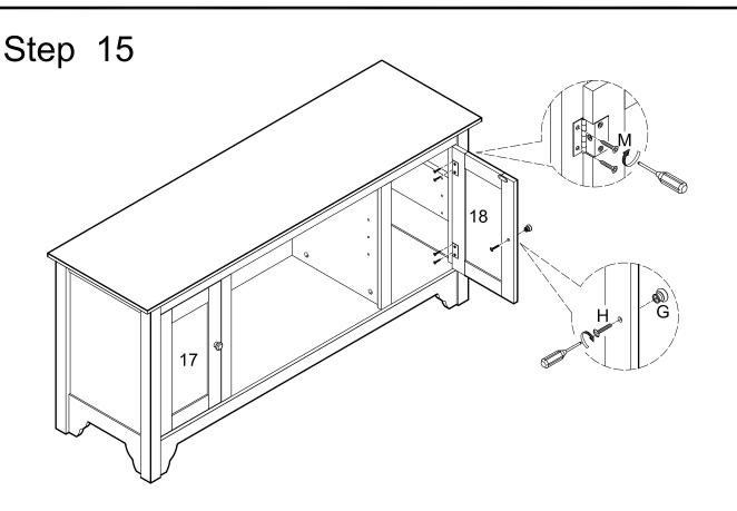
Attach doors (17,18) to the stand assembly using medium screws (M) at the hinges. Attach handles (G) to doors (17,18) using bolts (H).
