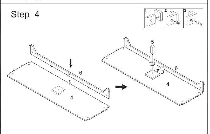
Attach slat (6) to bottom panel (4) using cam bolt and dowels as guides. Insert cam lock (D) into slat (6) and tighten with a screwdriver. Screw leg (5) into bottom panel (4).
