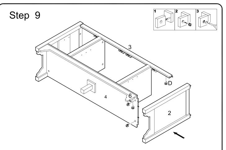
Attach side panel (2) to the opposite side of the assembly from Step 7 using cam bolts and dowels as guides. Insert cam locks (D) into bottom panel (4) and slats (3, 6). Tighten cam locks (D) with a screwdriver.
