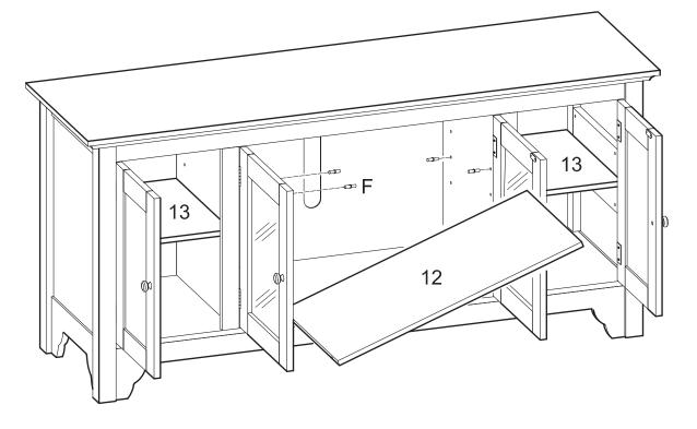
Insert shelf support pins (F) into the stand assembly at the desired shelf heights. Place shelves (12,13) on shelf support pins (F).
