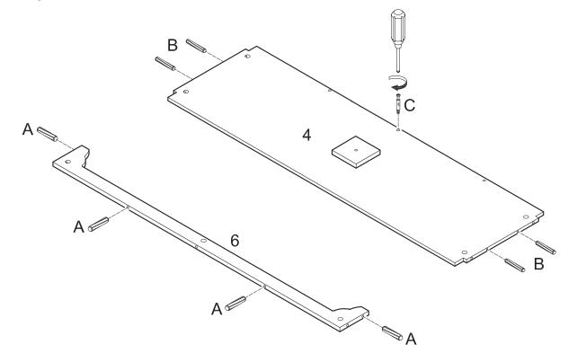
Insert large dowels (A) into slat (6). Insert small dowels (B) into bottom panel (4). Screw cam bolt (C) into bottom panel (4).
