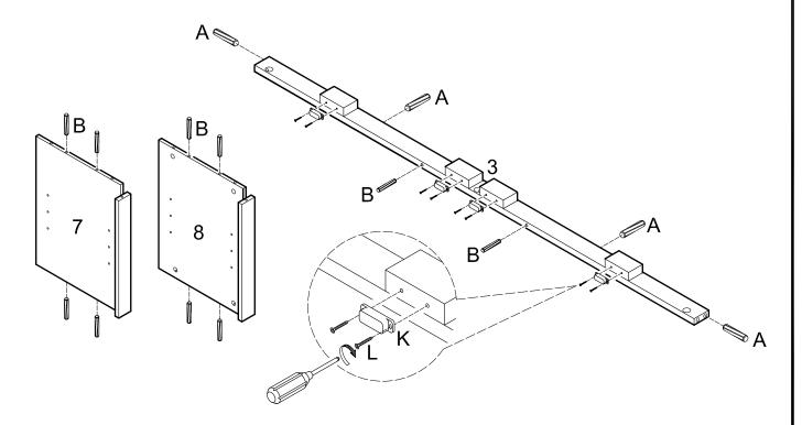
Insert small dowels (B) into panels (7,8) and slat (3). Insert large dowels (A) into slat (3). Attach door stoppers (K) to slat (3) using large screws (L).
