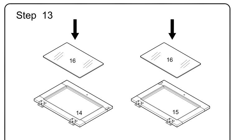
Attach glass panels (16) to door frames (14, 15) as shown in the diagram.
