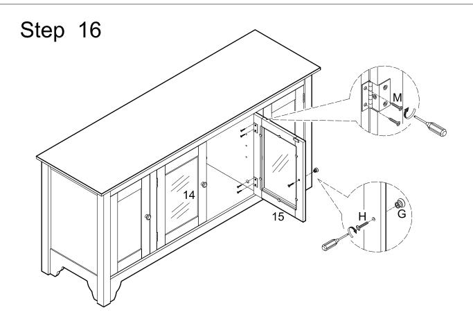
Attach doors (14,15) to the stand assembly using medium screws (M) at the hinges. Attach handles (G) to doors (14,15) using bolts (H).
