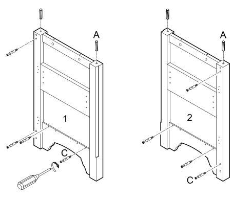
Insert large dowels (A) into side panels (1,2). Screw cam bolts (C) into side panels (1,2).
