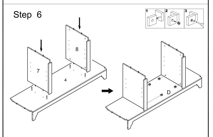
Attach panels (7,8) to bottom panel (4) using cam bolts and dowels as guides. Insert cam locks (D) into panels (7,8) and tighten with a screwdriver.
