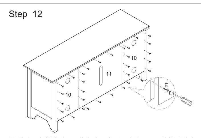
Attach back panels (10,11) to the assembly from the previous step using flange screws (E). *Note that back panels (10) will overlap back panel (11).*
