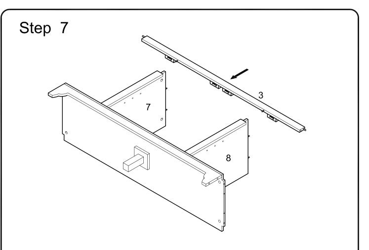
Attach slat (3) to the assembly from the previous step using dowels as a guide.
