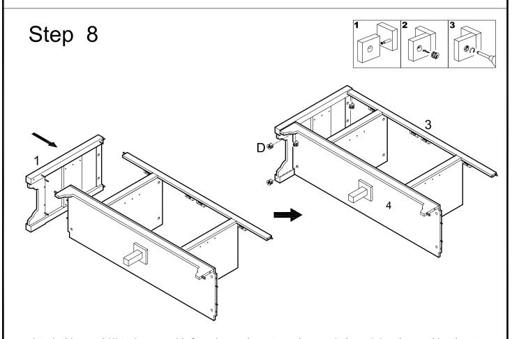
Attach side panel (1) to the assembly from the previous step using cam bolts and dowels as guides. Insert cam locks (D) into bottom panel (4) and slats (3,6). Tighten cam locks (D) with a screwdriver.
