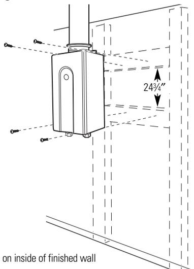
Boards on inside of finished wall
