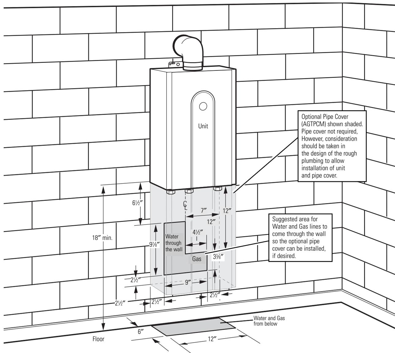
The center of the pipes can be placed anywhere within the shaded area. The center of the pipes is recommended to be protruding only within 6" of the mounting wall. Other specific installations may be different.
