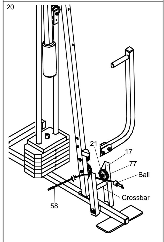
21. Route the Short Cable (58) around the 3 1/2" Pulley (15) attached to the lower hole in the Front Upright (42). **See the inset drawing. Be sure that the Cable Trap (66) is turned to hold the Cable in place and that the Cable is routed around the Pulley as shown.** Tighten the 3/8" Nylon Locknut (21) and the 3/8" x 3 3/4" Bolt (71).
