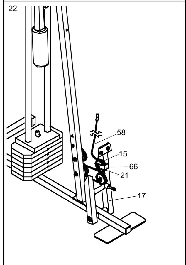
23. Route the Short Cable (58) around the 3 1/2" Pulley (15) attached to the upper hole in the Front Upright (42). **See the inset drawing. Be sure that the Cable Trap (66) is turned to hold the Cable in place and that the Cable is routed around the Pulley as shown.** Tighten the 3/8" Nylon Locknut (21) and the 3/8" x 3 3/4" Bolt (71).
