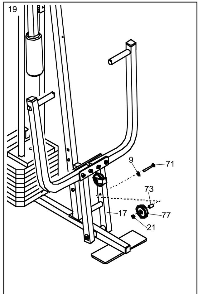
20. **Locate the Short Cable (58).** Route the Short Cable (58) under the 3 1/2" Low Pulley (77). **Be sure that the end of the Cable with the ball is on the indicated side of the Press Frame (17) and that the Cable is between the Pulley and the crossbar on the Press Frame.** Tighten the 3/8" Nylon Locknut (21) and the 3/8" x 3 3/4" Bolt (not shown).
