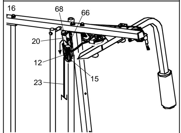
Be sure that the 5/16” x 5” Bolt (68) is properly tightened and that the Pulley Bracket (20) can move freely.
