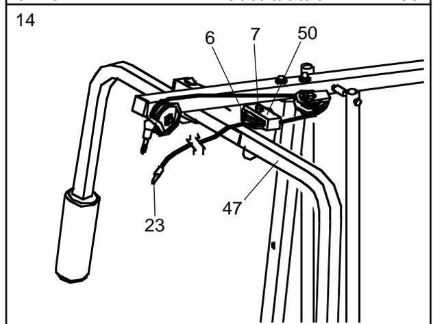
15. Route the Long Cable (23) around the “V”-Pulley (6) on the Right Arm (48). **Be sure that the Cable is in the groove of the “V”-Pulley and that the Long Cable Trap (50) is turned to hold the Cable in place.** Tighten the 3/8” x 2 1/2” Bolt (7) and the 3/8” Nylon Locknut (not shown).
