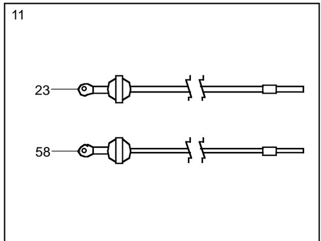
12. **Locate the Long Cable (23).** Route the Long Cable around the indicated 3 1/2" Pulley (15) attached to the Top Frame (55). **Be sure that the end of the Cable with the ball is on the indicated side of the Pulley and that the Cable is between the Pulley and the hook.** Tighten the 3/8" x 3 3/4" Bolt (71) and the 3/8" Nylon Locknut (not shown).
