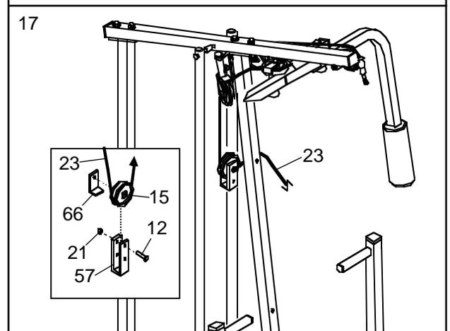
Route the Long Cable (23) around the 3 1/2” Pulley (15) and through the Long “U”-Bracket (57). **Be sure that the Cable is in the groove of the Pulley and that the Cable and Pulley move smoothly.**
