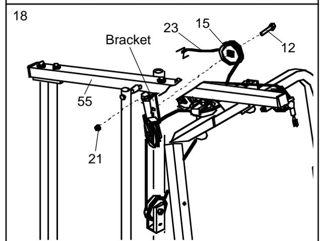
Route the Long Cable (23) around the 3 1/2” Pulley (15) attached to the bracket on the Top Frame (55). Tighten the 3/8” x 2” Bolt (12) and the 3/8” Nylon Locknut (21). **Be sure that the Cable is in the groove of the Pulley and that the Cable and Pulley move smoothly.**
