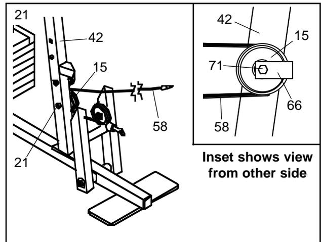
22. Route the Short Cable (58) around the 3 1/2" Pulley (15) attached to the upper hole in the Press Frame (17). **Be sure that the Cable Trap (66) is turned to hold the Cable in place and that the Cable is routed around the Pulley as shown.** Tighten the 3/8" Nylon Locknut (21) and the 3/8" x 3 1/2" Bolt (not shown).
