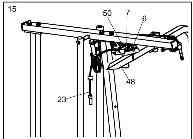
16. Route the Long Cable (23) around the 3 1/2” Pulley (15) attached to the Pulley Bracket (20). **Be sure that the Cable is in the groove of the Pulley and that the Cable Trap (66) is turned to hold the Cable in place.** Tighten the 3/8” x 2” Bolt (12) and the 3/8” Nylon Locknut (not shown).
