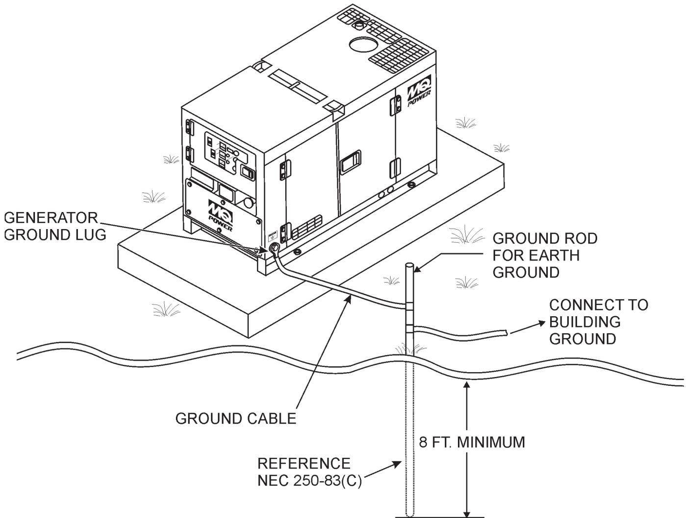
Figure 4. Typical Generator Grounding Application
