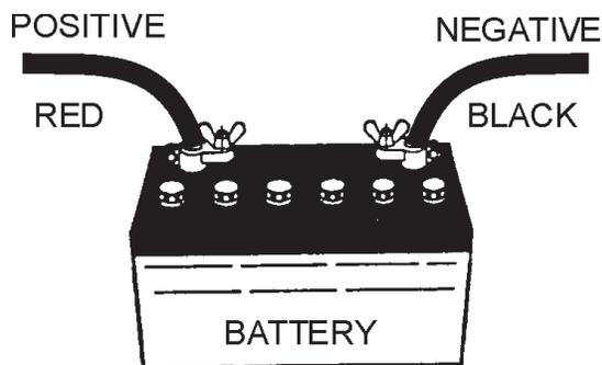
Figure 37. Battery Connections
