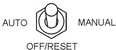
**Figure 57. MPEC Control Switch (Off/Reset)**
