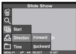
**7 Press the ▲ or ▼ key so that the desired direction is highlighted and press ► to finish the setting.**
