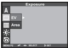
**3 Press the ▲ or ▼ key so that [EV] is highlighted and press the ► key.**
