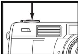
**4 Press the shutter-release button half-way down.**
