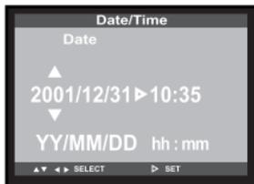
**4 Press the ▲ or ▼ key to specify or correct the date and press ► key to finish the setting.**
