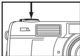
**6 Press the shutter-release button full-way down to take picture.**
