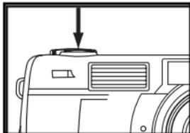
**5 Press the shutter-release button full-way down to take a picture.**
