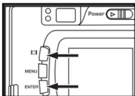
**4 When the selected image is highlighted, press the LCD to select, then press the ENTER button.**
