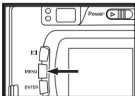
**1 Rotate the function dial to
