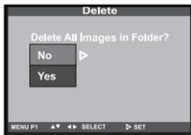
**6 Press ▼ key so that [YES] is highlighted and press ► key to finish the Deleting.**
