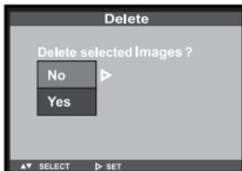
**8 Press the ENTER button so that [YES] is highlighted, and press
