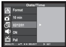
**2 Press the ▲ or ▼ key so that [DATE/TIME] is highlighted and press the ► key.**
