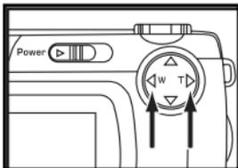
**4 Adjust the image range and size with the four-way keys (◀ / ▶).**
