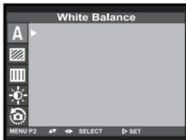
**2 Press the ▲ or ▼ key so that [White Balance] is highlighted and press the ► key.**
