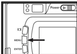
**1 Rotate the function dial to
