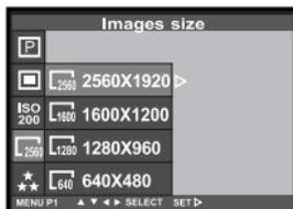
**3 Press the ▲ or ▼ key so that the desired image size mode is highlighted and press the ► key.**
