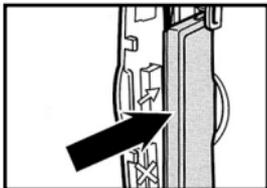
**2 Insert the CF card into the card slot.**
