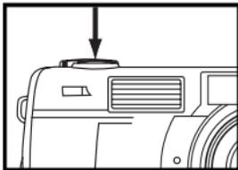
**6 Press the shutter-release button full-way down to take the picture.**
