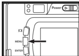
**1 Rotate the function dial to
