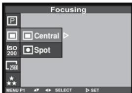
**3 Press the ▲ or ▼ key to select desired focus area and press ► key to finish the setting.**
