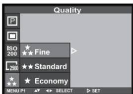
**3 Press the ▲ or ▼ key so that the desired image quality mode is highlighted and press ► key to finish the setting.**
