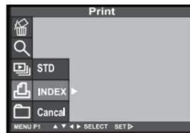
**3 Press the ▼ key so that [INDEX] is highlighted and press
