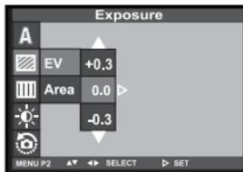
**4 Press the ▲ or ▼ key that the desired exposure compensation value and press ► to finish the setting.**
