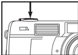
**5 Press the shutter-release button full-way down to take the picture.**
