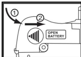
**4 Close the battery-chamber door in the direction of the arrow ① and slide it until it clicks ② .**
