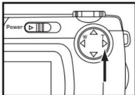
**9 To complete the operation of deleting an image, after confirming that [NO] is highlighted in the display to confirm, press the
