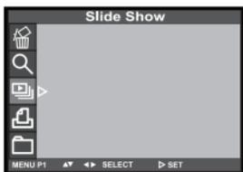
**2 Press the ▲ or ▼ key so that [SLIDE SHOW] is highlighted and press
