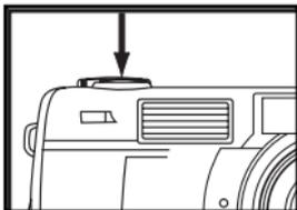
**5 Press the shutter-release button half-way down.**
