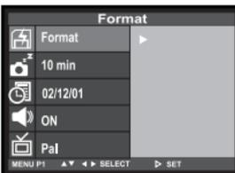
**3 Press the ▲ or ▼ key so that [FORMAT] is highlighted and press ► key.**
