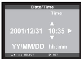
**7 Press the ▲ or ▼ key to specify or correct the date and press the ► to finish the setting.**
