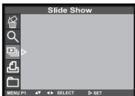
**2 Press the ▲ or ▼ key so that [SLIDE SHOW] is highlighted and press ► key.**
