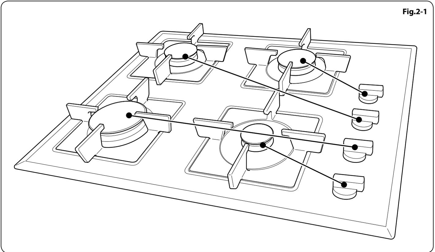
The diagram by each of the control knobs indicates which burner that knob operates (**Fig.2-1**). Each burner has a special Flame Safety Device (FSD) that stops the flow of gas if the flame goes out.
