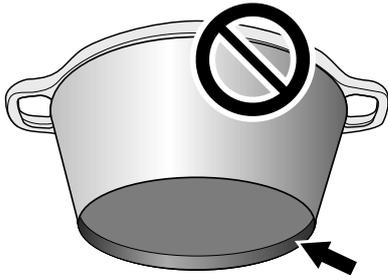
Pans and kettles with concave bases or down turned base rims should not be used (**Fig.2-5**).
