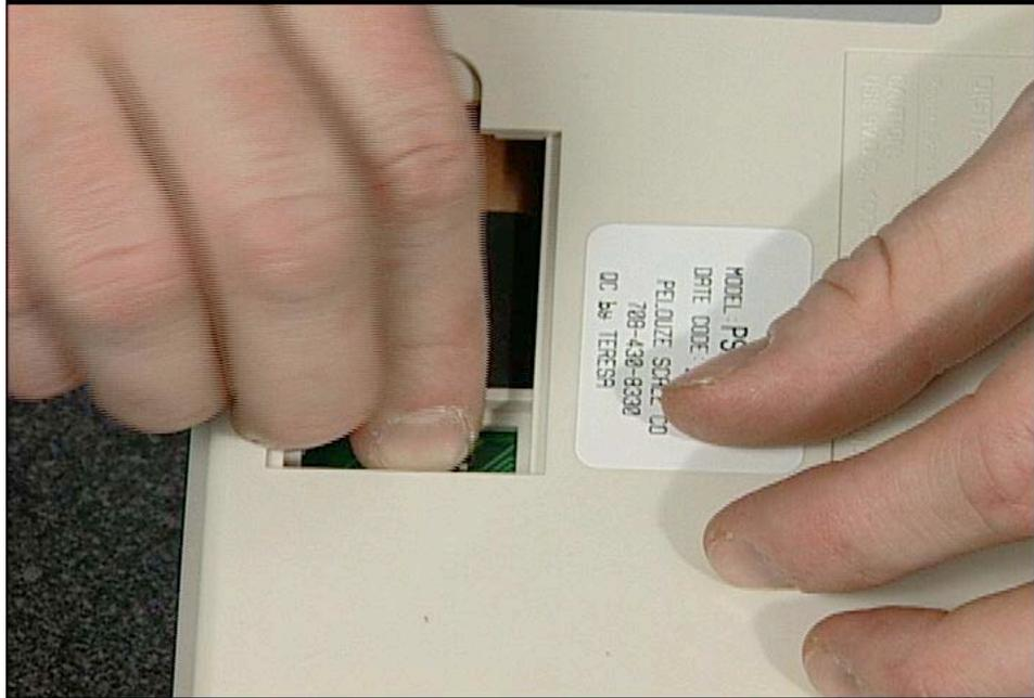
Gently press down to seat the chip into the socket.
