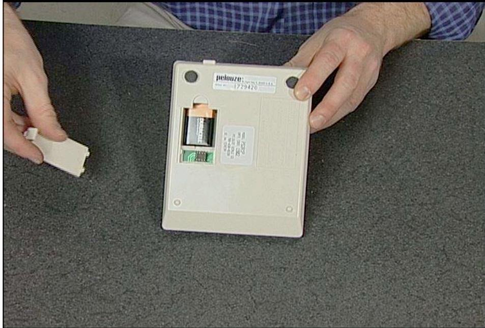
Remove the battery rate chip compartment cover from the bottom of the scale.
