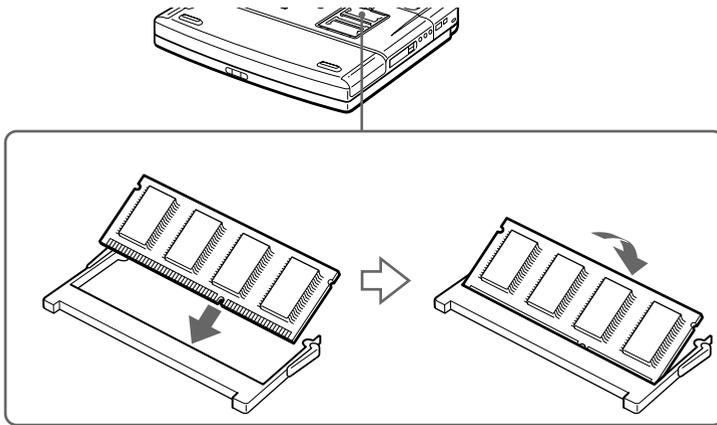
1 Slide the memory module into the slot.
