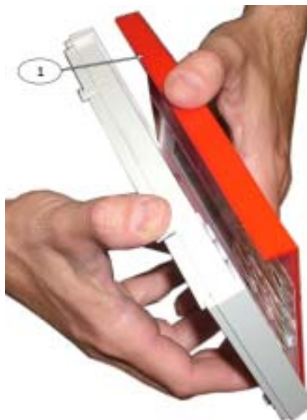
Figure 5: Lifting the Red Cover
