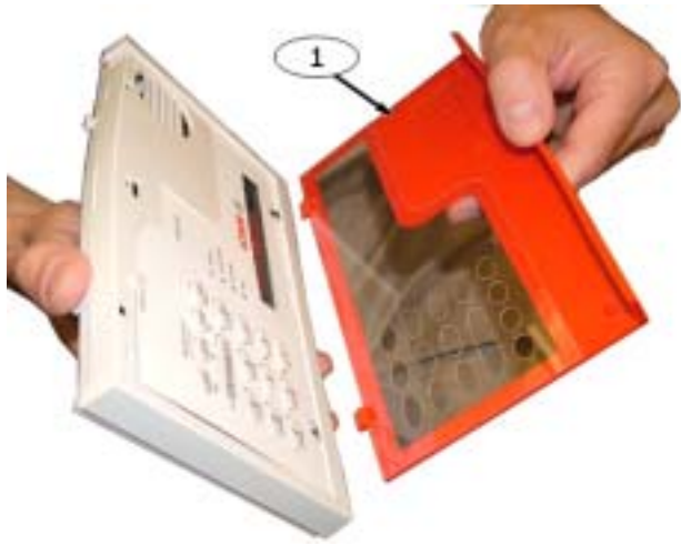
Figure 6: Removing the Red Cover
