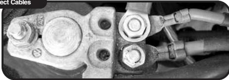
You might observe a spark when you make this connection since current can flow to charge capacitors in the inverter.
