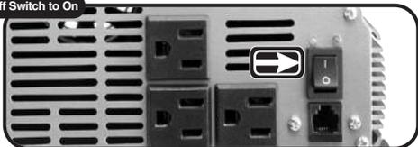
The inverter is now ready to deliver AC power to your loads. If several loads are to be operated by the inverter, turn them **on** separately, after the inverter has been turned **on**. This will ensure that the inverter does not have to deliver the starting currents required for all the loads at once.
