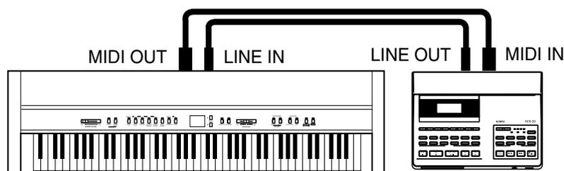
Next you must match the MIDI channel. The transmitting channel of the CE200 piano and receiving channel of your external MIDI device must be the same.
