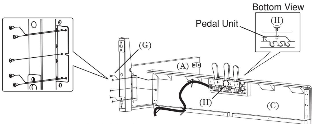
1. Insert the Adjuster (H) on the Pedal Unit.
