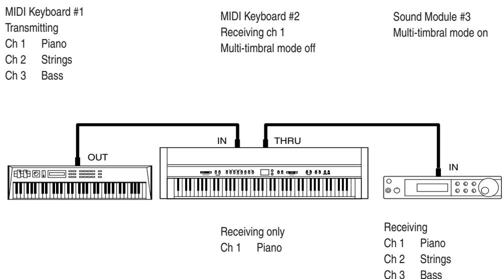
Instrument #2 recognizes only the piano part received from Instrument #1. Instrument #3 receives all the parts on the three channels being passed through Instrument #2 because Instrument #3's multi-timbral mode capability is activated.
