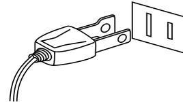
It is a good practice to have the instrument near the AC outlet and the power cord plug in a position so that it can readily be disconnected in an emergency because electricity is always charging while the plug is in the AC outlet even in a power switch off condition.
