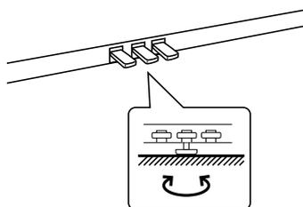
**11.** Turn the adjuster (installed on the bottom of the Pedal Unit) down until it makes firm contact with the floor. If the floor is carpeted, place a spiked furniture cup under the adjuster so that it makes firm contact with the carpet backing. Press any pedal with your foot. If the pedal rail flexes, lower the adjuster until flexing is minimized.
