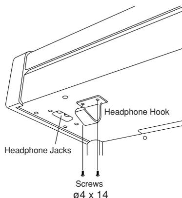
**1.** Attach the Headphone Hook with two screws (ø4 x 14) to the holes next to the headphone jacks.
