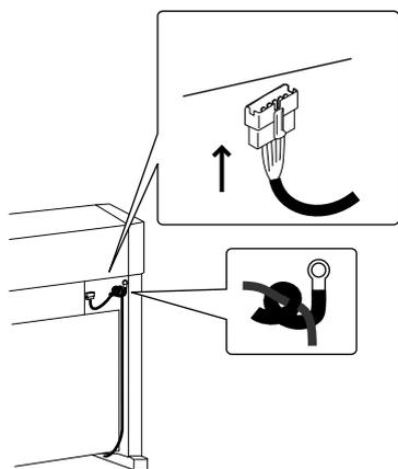
**10.** Insert the pedal connection cord that comes from Pedal Board into the main unit's pedal jack and fix with the clamp of the Side Panel.
