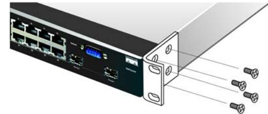
**Figure 3-2: Attach the Brackets to the Switch**
