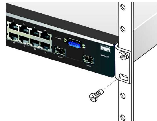
**Figure 3-3: Mount the Switch in the Rack**
