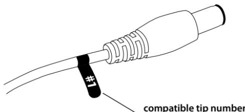
3. Attach the selected connector to the end of the output cable of the AC adaptor.
