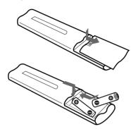
Insert the negative (–) end first, then push in and down until the positive (+) end clicks into position. When you close the compartment lid, make sure to fix its position first.
