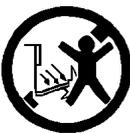
Stand clear when opening the drop down oven door. **Do not** allow it to fall open - support it using the door handle, until it is fully open.
