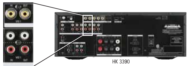
Figure 15 – Video 1 A/V Inputs and Outputs
