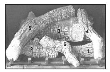
**STEP 7:** (SRV2057-725): Place log 6 on log 2 as shown. The left end of log 6 should touch the upper knot of log 2. The right end of log 6 should rest on the grate bar, centered between tine 4 and 5. NOTE: The front faces (C) of log 6 and 2 should be on the same plane. This is key in avoiding flame impingement.
