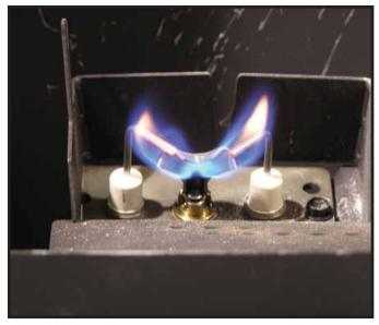
Figure 3.1 IPI Pilot Flame Patterns
