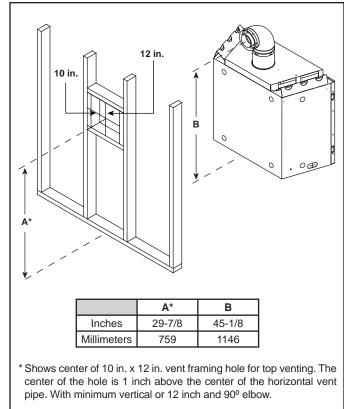
Figure 8.6 Wall Penetration
