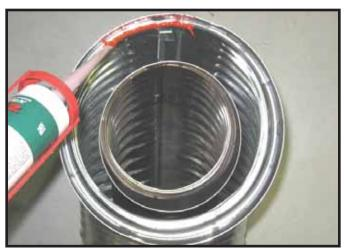
Figure 10.1 High Temperature Silicone Sealant
