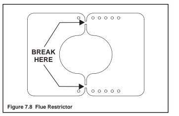
3. Match the amount of vertical in the system with the chart to find the appropriate position to set the Flue Restrictor (see Figure 7.9).
