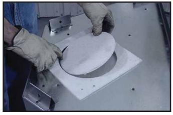
Figure 9.2 Remove the center insulation plug.
