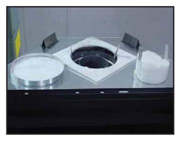
**Figure 9.5** Discard the seal cap, remove and discard the insulation basket. Note: Once the vent cap has been removed it cannot be reattached.
