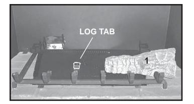
**STEP 2:** Log #1 (SRV2057-720): Place log 1 so that the bottom right notch on log rests on far right grate tine. The bottom left notch on log #1 must mate over the log tab on the burner face.
