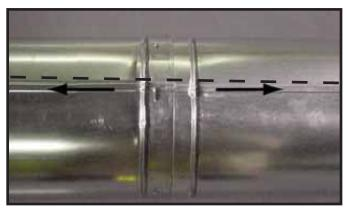
Figure 10.11 Align and Disassemble Vent Sections
