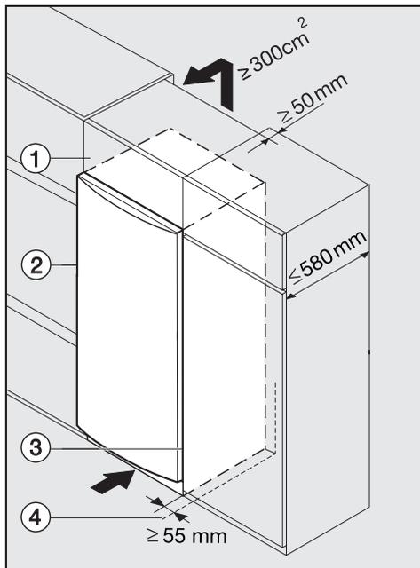
The air inlet and outlet must not be covered or blocked in any way. They should be dusted on a regular basis.
