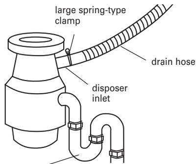
3. Insert drain hose through hole cut in cabinet to the front center of opening where drain connection will be made.
