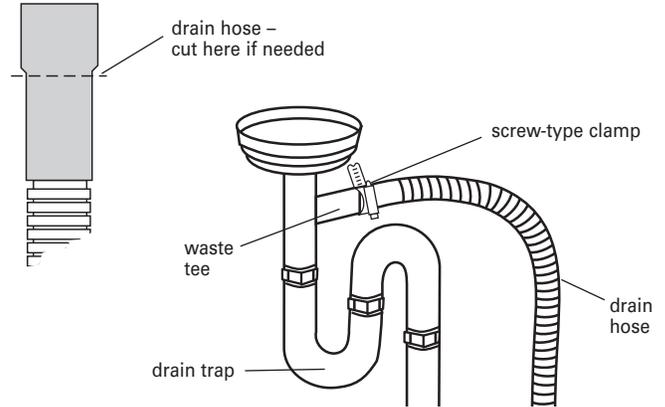
3. Insert drain hose through hole cut in cabinet to the front center of opening where drain connection will be made.
