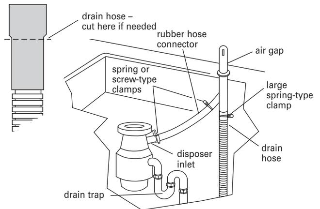
4. Insert drain hose through hole cut in cabinet to the front center of opening where drain connection will be made.
