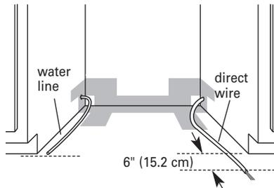
If the water line and the direct wire reach far enough into the opening, proceed to the next section "Install the drain hose." If they do not reach far enough, follow the steps under "Prepare cabinet opening where there are no existing utility hookups."
