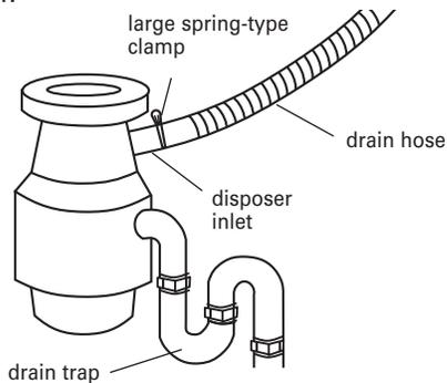
3. Insert drain hose through hole cut in cabinet to the front center of opening where drain connection will be made.
