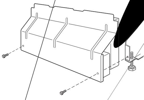
5. Check that the screws are tight and that the contacts of the lower panel are in contact with the dishwasher leg.
