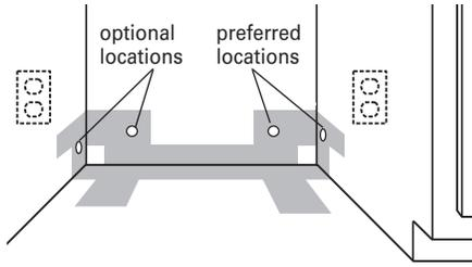
Metal cabinet: Cover hole with grommet (Part No. 302797) included with power supply cord kit.
