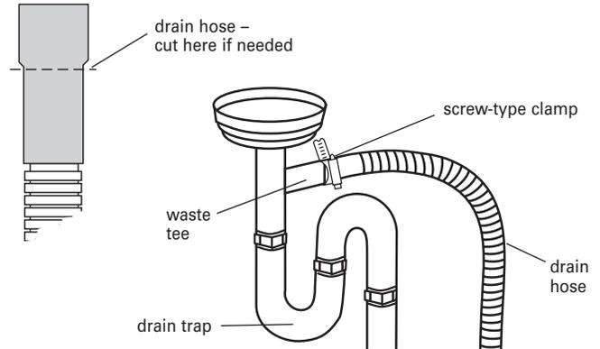
3. Insert drain hose through hole cut in cabinet to the front center of opening where drain connection will be made.
