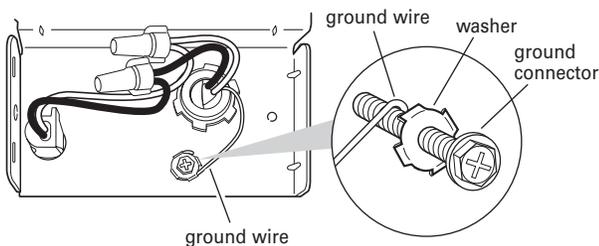
6. Tighten clamp connector or conduit connector screws.
