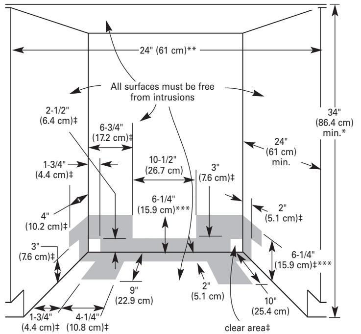
Cut holes in shaded area of cabinet walls or floor as specified below:
