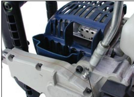
Figure 20 Gearcase Grease Fitting
