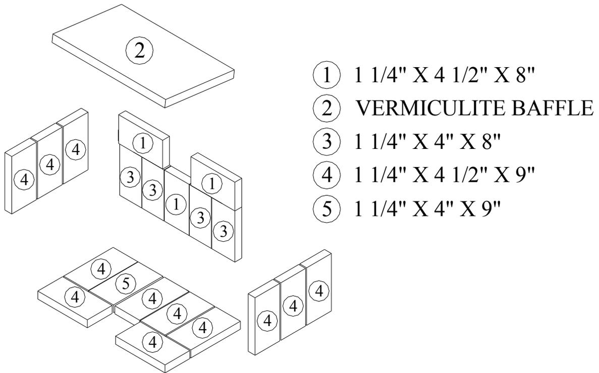
**Figure 4.6.1 (B) - Firebrick layout for Escape 1800 model**
