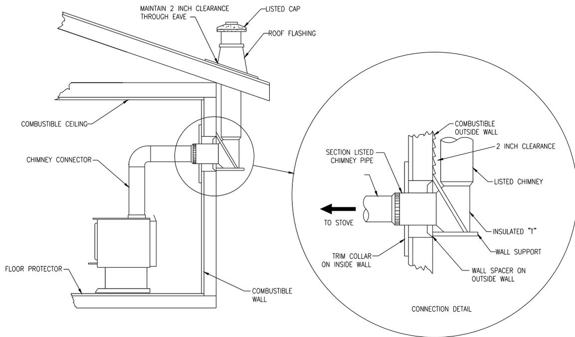
**FIGURE 2.2.1 (A) Typical installation through the wall**
