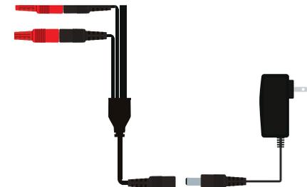
**STEP 3.** Connect the power lead on the power splitter to the camera power adapter. **DO NOT** plug the adapter into an outlet at this time.
