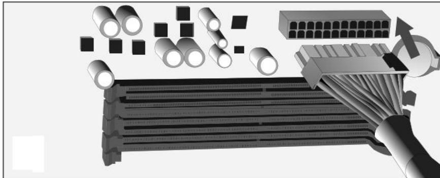
3. Connect the 8-pin or 4+4-pin connector for the CPU. If your motherboard has an 8-pin socket with a cover on some of the openings, we recommend that you remove the cover and use the 8-pin connector.
