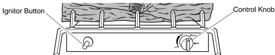
Figure 21 - Control Knob and Ignitor Button Location
