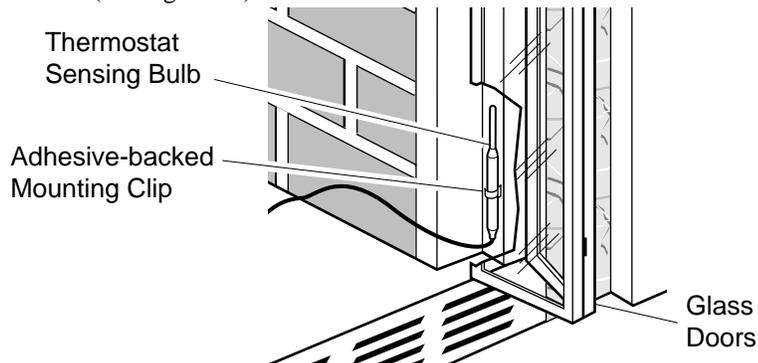
**Figure 32 - Installing Thermostat Sensing Bulb behind Glass Doors**
