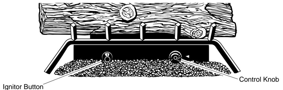
*Figure 23 - Control Knob and Ignitor Button Location*
