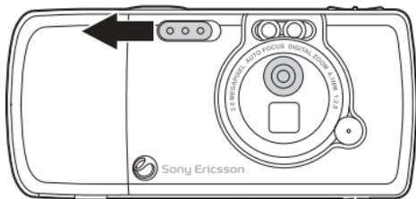
While in standby, slide the lens cover lock to activate the camera.
