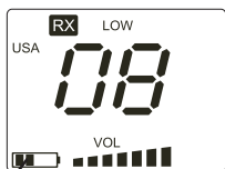
Battery Level Indicator
