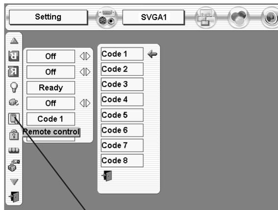
When pressing SELECT button at Remote control, Remote control code Menu appears.
