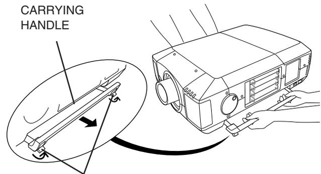
Pull up lock buttons to release lock.
