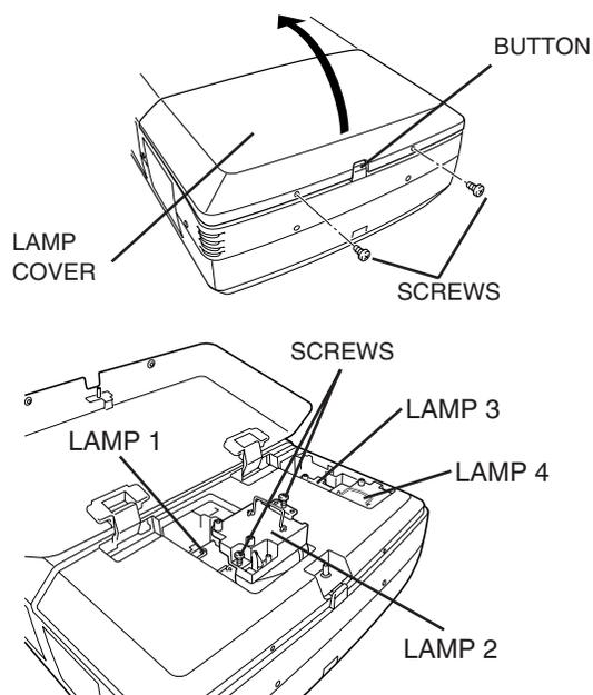
Make sure which number of lamp needs to be replaced on Lamp Status Display. Figure shows case of replacing LAMP 2.
