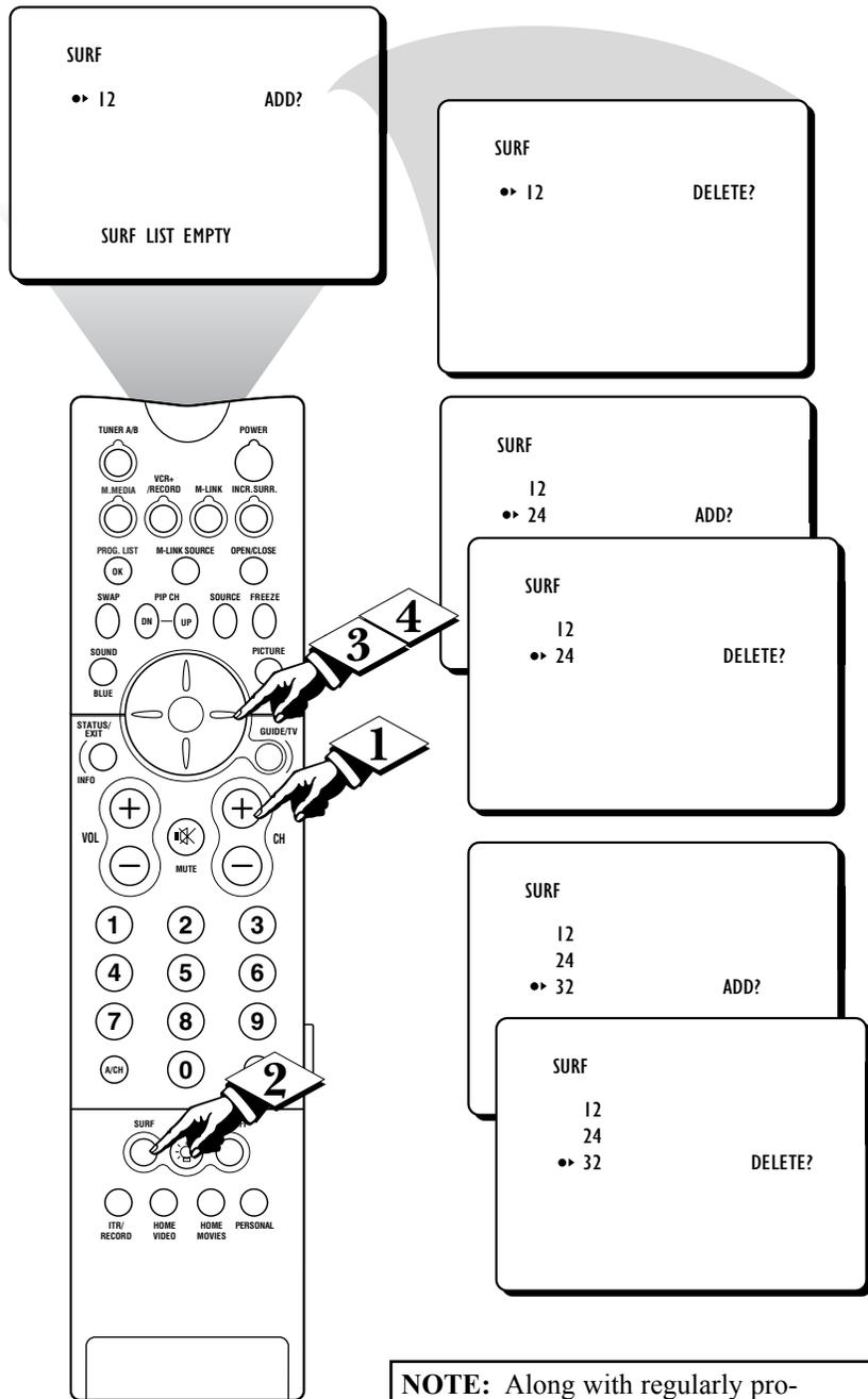
**NOTE:** Along with regularly programmed channels, the external video source connections can be added to the SURF list. This means that the AV1, AV2, and AV3 channels can be added to your SURF list. Just tune to their channel and use the same procedure described on this page.
