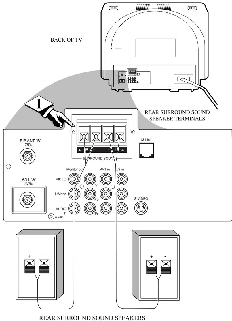
**NOTE:** The rear speakers are intended to give a background noise effect that requires a lower volume level than the TV's front speakers. The volume level being heard from these speakers will be lower than the volume level being heard at the front TV speakers
