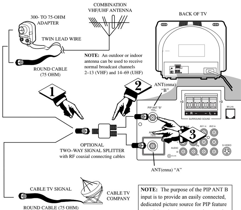
**NOTE:** The purpose of the PIP ANT B input is to provide an easily connected, dedicated picture source for PIP feature use. Other signal source options (such as a satellite dish system, an additional external antenna, a VCR, or a video game) also could be connected and displayed on the TV's PIP screen window through the use of the PIP ANT B input.
