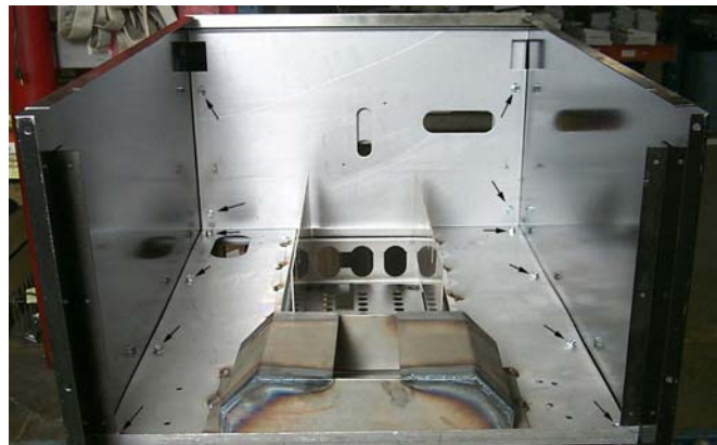
Remove screws (arrows) securing the firebox to the cabinet.
