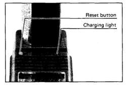
charging light goes out within 10 seconds even after pressing the reset button a couple of times, the battery cartridge is dead. (CAUTION: Wait for more than 5 seconds after the charging light goes out to press the reset button again.) Replace it with a new one. When the charging light goes out after about one hour, you may remove the fully charged battery cartridge. After charging, unplug the charger from the power source.
