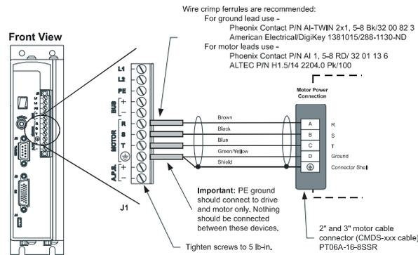
Figure 14: Epsilon Motor Power Wiring Diagram
