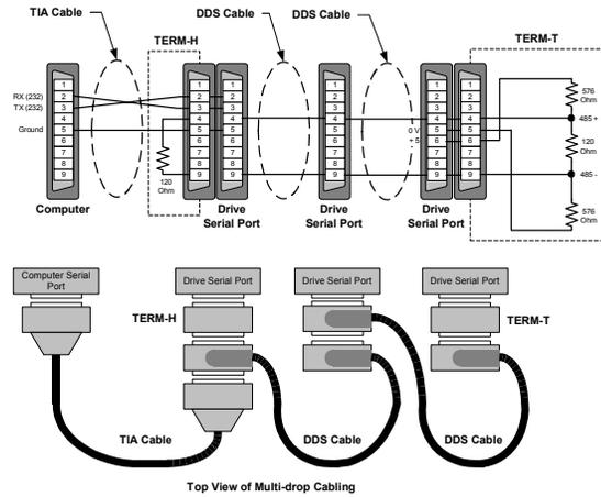
Figure 32: Multi-Drop Wiring Pinout
