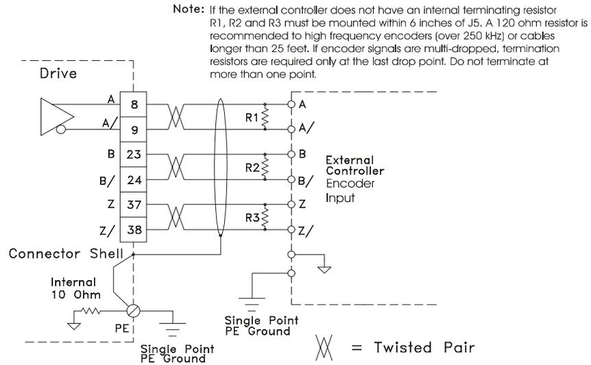
Figure 23: Command Connector Encoder Output Wiring
