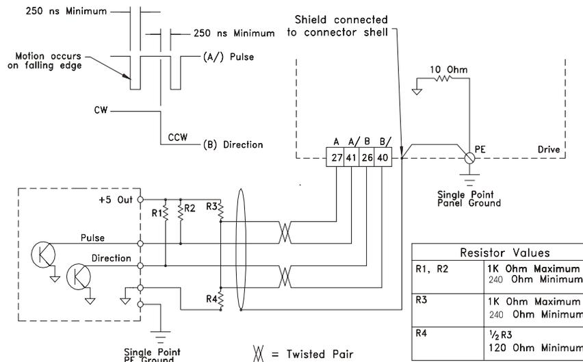
Figure 26: Pulse Mode, Single Ended Output to Differential Input
