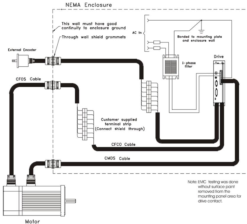
Figure 3: AC Filter and Cable Connections for Epsilon Drives
