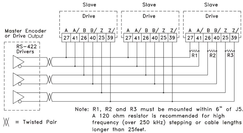
Figure 29: Master/Slave Encoder Connections
