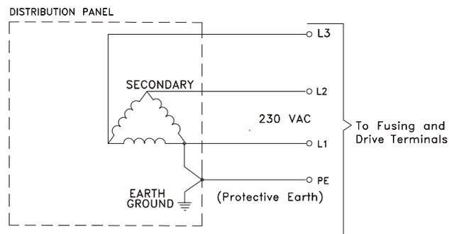
Figure 6: Earth Grounded Delta Distribution Transformer
