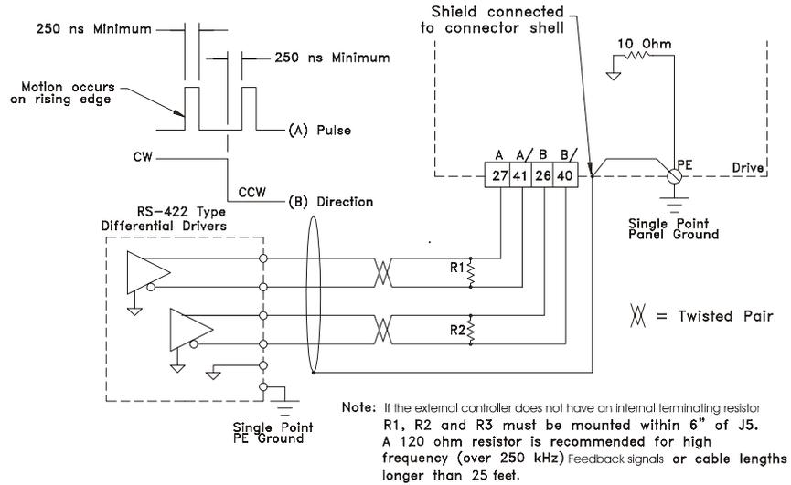
Figure 25: Pulse Mode, Differential Output to Differential Input
