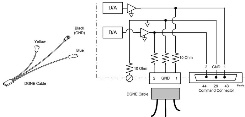
Figure 33: Diagnostic Cable (DGNE) Diagram
