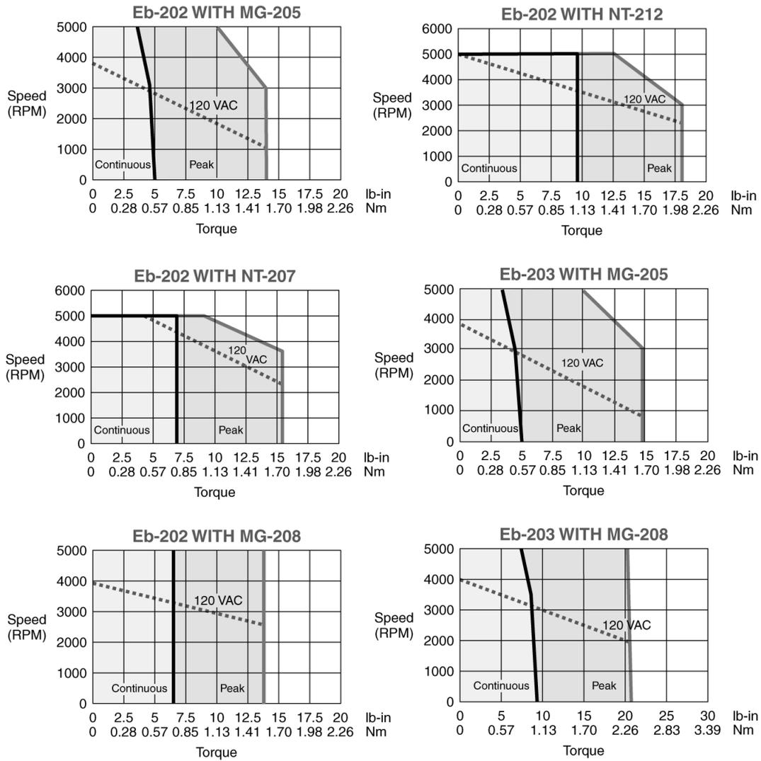
Figure 43: Epsilon Speed Torque Curves, sheet 1 of 2
