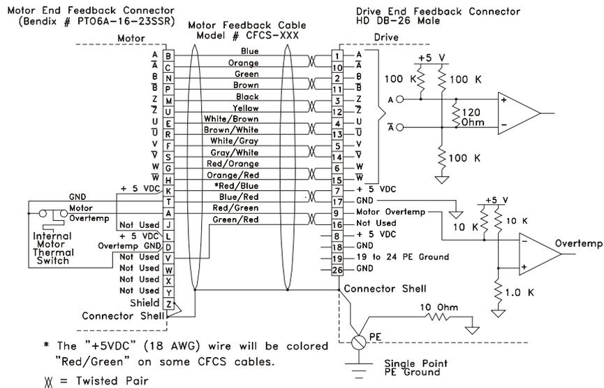
Figure 15: Motor Feedback Connector Pinout
