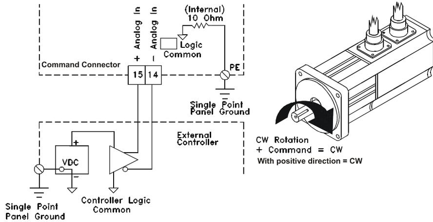
Figure 21: Analog Command, Differential Wiring Diagram
