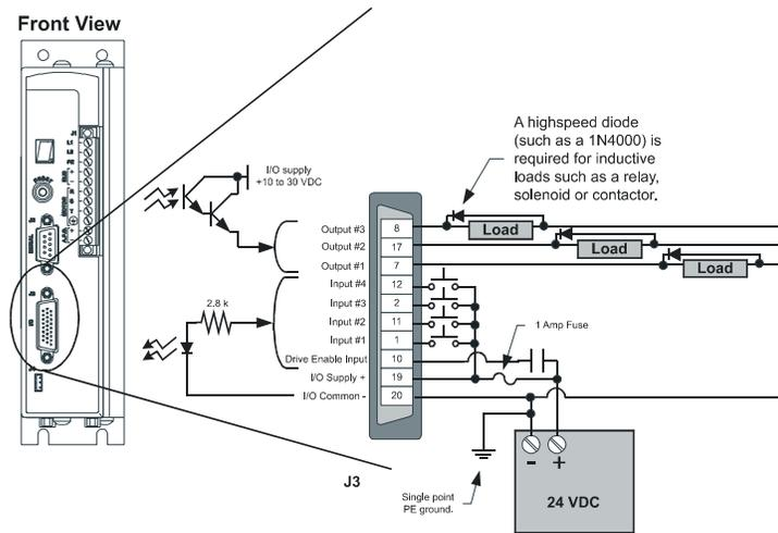
Figure 18: Epsilon Input/Output Wiring Diagram
