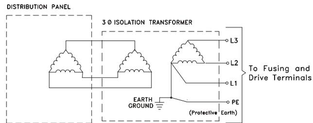
Figure 9: *Delta to Delta Isolation Transformer*
