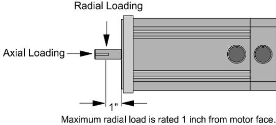
Figure 42: Axial/Radial Loading
