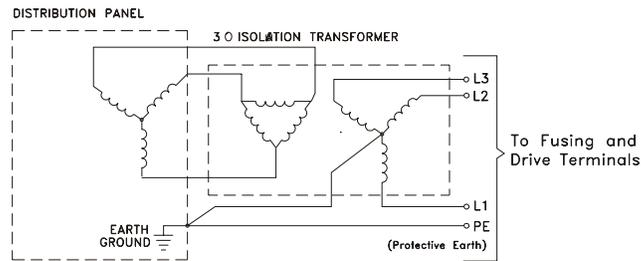
Figure 8: *Three Phase WYE (ungrounded) Distribution to a Three-Phase Delta/WYE Isolation Transformer*
