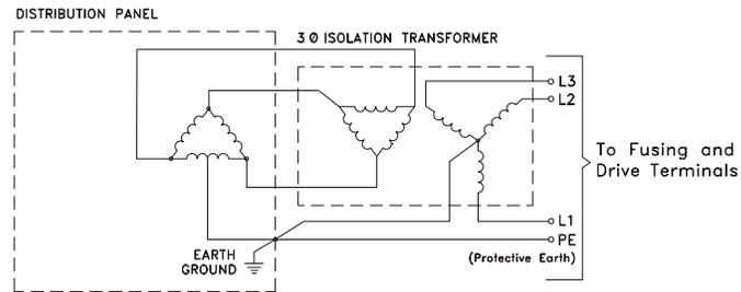
Figure 7: *Three Phase Delta (with mid-phase GND) Distribution to a Three-Phase Delta/WYE Isolation Transformer*
