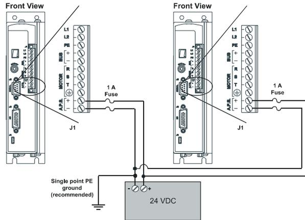
Figure 13: Multiple APS Wiring Diagram
