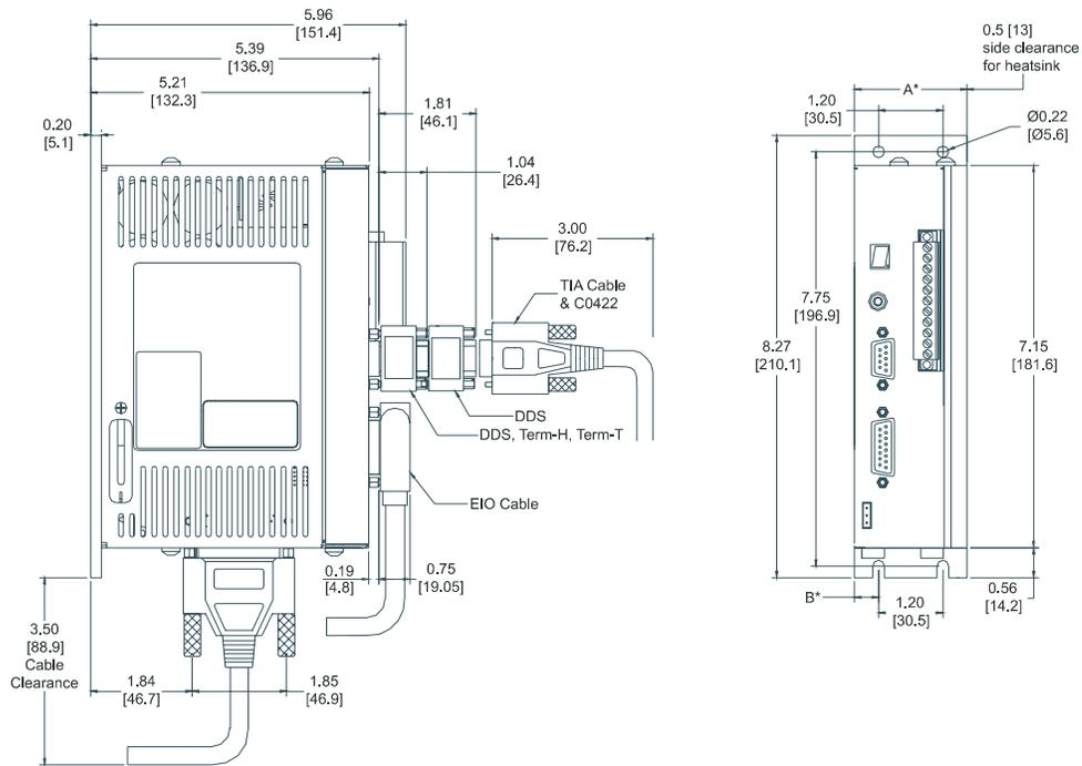
Figure 45: Drive Dimensions Eb-202, Eb-203, Eb-205
