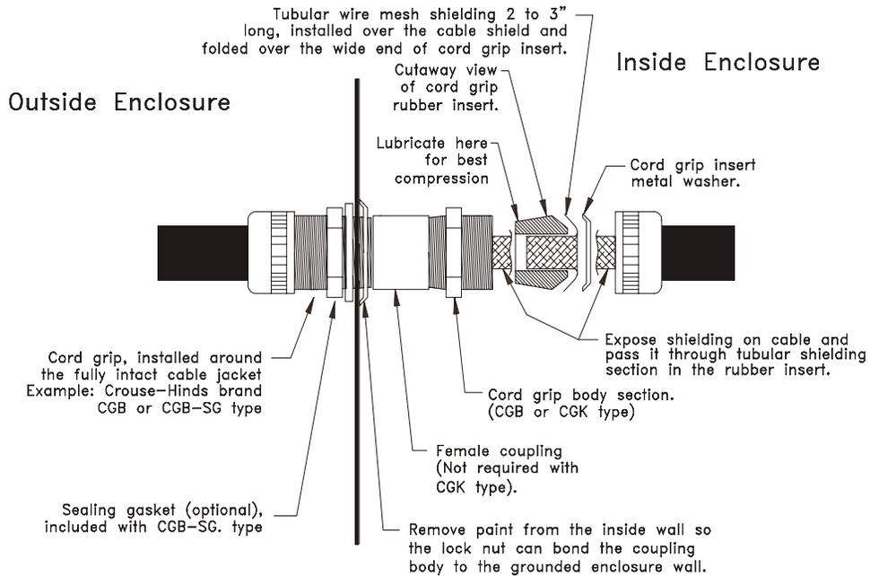
Figure 2: Through Wall Shield Grommet
