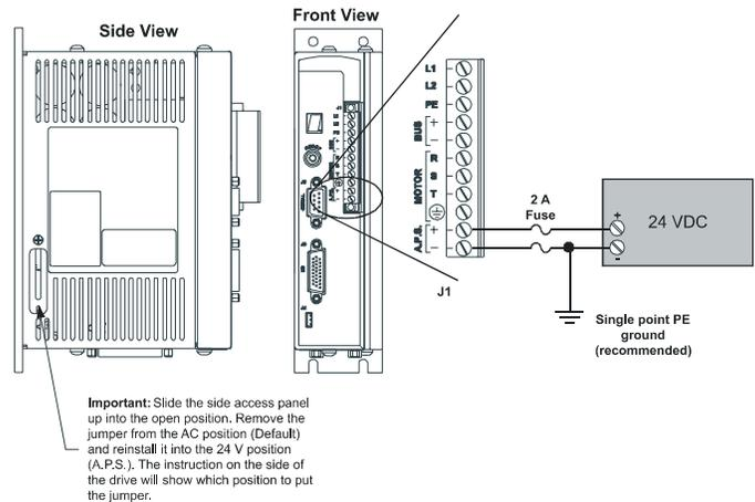
Figure 12: Epsilon Auxiliary Power Supply Wiring Diagram
