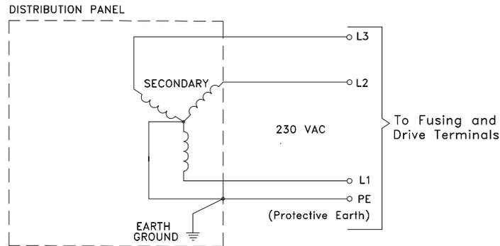
Figure 5: Earth Grounded WYE Distribution Transformer
