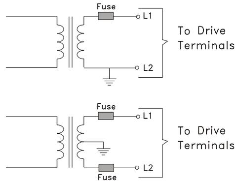
Figure 10: Single Phase Power Supply Connections
