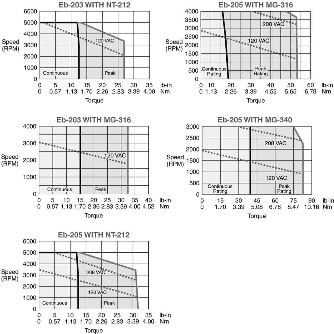
Figure 44: Epsilon Speed Torque Curves, sheet 2 of 2
