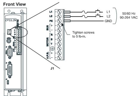
Figure 11: Epsilon AC Power Wiring Diagram
