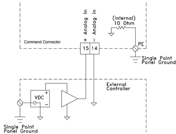
Figure 22: Analog Command, Single Ended Wiring Diagram
