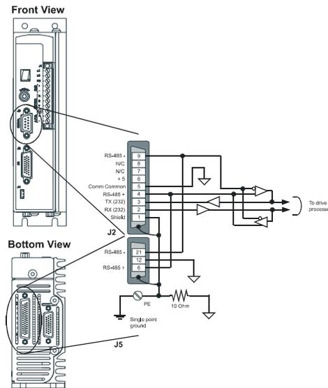
Figure 30: Epsilon RS-232 and RS-485 Internal Connections between the Command Connector and the Serial Communication Connector
