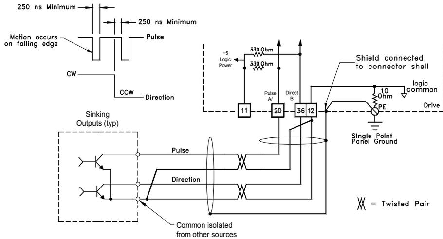
Figure 27: Pulse Mode, Single Ended Output to Single Ended Input (twisted pair cable)
