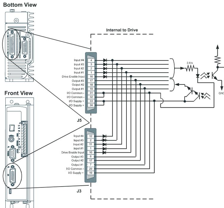
Figure 19: Epsilon I/O to Command Connector Internal Connections
