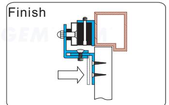
Finish Once the position is correct, use the screws to permanently mount the Z bracket on the door frame. This should be the last step.
