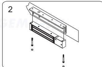
2 Tighten the electromagnetic lock on the L bracket by using the fixing screw.
