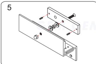
5 Put one rubber washer between armature plate and the Z bracket.
