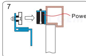
7 Turn on the power of EM-Lock, and let the armature plate bonds to the EM-lock. Adjust the position between the Z bracket and the door frame.
