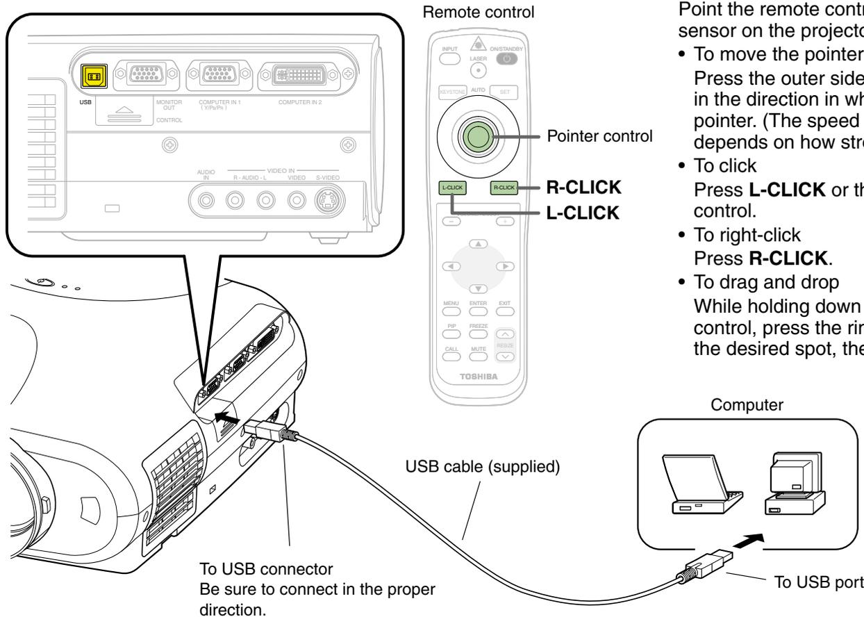
Point the remote control at the remote control sensor on the projector when operating its buttons.
