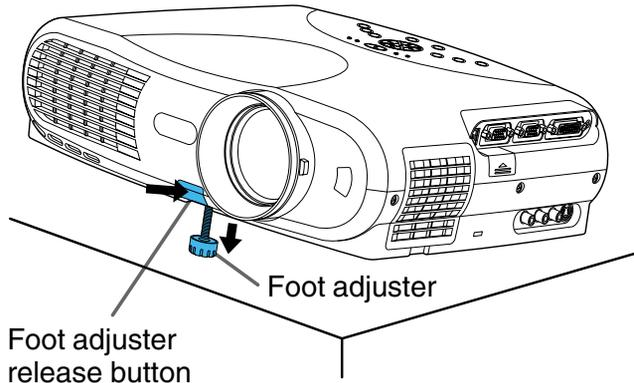
**Lift the front of the projector until the desired tilt angle is obtained and hold down the foot adjuster release button.**
