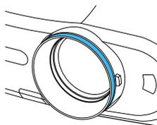
**Focus on the picture by turning the focusing ring.**
