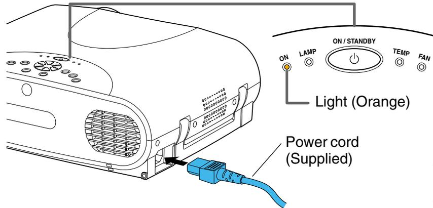
The three indicators, TEMP, LAMP, and ON, light in green for several seconds and then the ON indicator lights in orange and the projector turns to the standby mode.
