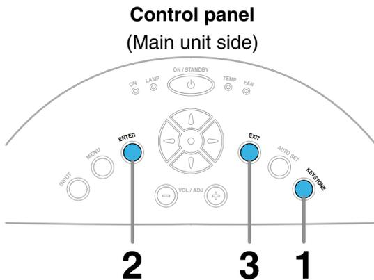
A picture may be expanded on the upper side if projected upward from the projector lifted up by the foot adjuster. The projector can correct this keystone distortion.
