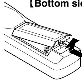
**【Bottom side】****Open the cover.****2**
