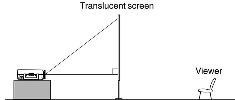
**1 Place the projector on a steady, level surface such as a table.**
