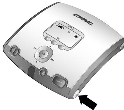
When you turn on your PCD-1, the LCD screen briefly displays **Compaq iPAQ PCD-1**, followed by the message “Reading Disc.” If there is no disc loaded, you will receive the message “No Disc.” If a disc is loaded, you will receive the message “Searching for audio.” If audio files are present, the PCD-1 will list the number of tracks found then begin playing the first track. If no audio tracks are found, it will display the message “No Audio Found.”
