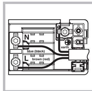
3. Remove the wire contact screws L-N- $\perp$ , then fasten the wires under the screw heads, respecting the colour code: Black/Blue (N), Red/Brown (L) and Bare Wire/Yellow-Green ( $\perp$ ).
