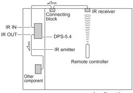
Connect the IR emitter to the DPS-5.4's IR OUT, and place the IR emitter in front of the other AV component's remote control sensor (usually located on its front panel), as shown below. See the instructions supplied with the IR emitter.
