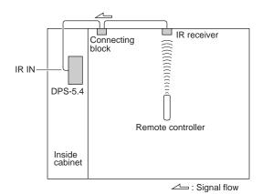
Connect the IR receiver to the DPS-5.4 as shown below.
