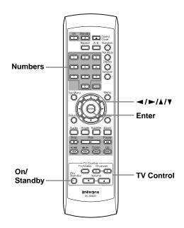
You can make RC-536DV remote controller to operate a TV from other brand than Integra/Onkyo by storing the pre-programming code of the brand in the RC-536DV.
