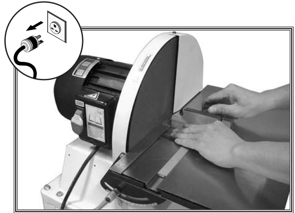
Figure 18. Squaring miter gauge to disc.
