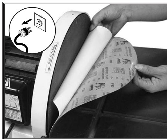
Figure 12. Sandpaper being slipped between the disc and table.
