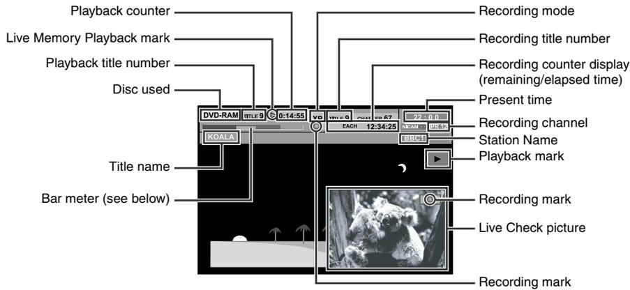
This unit displays the current recording/playback status by the bar meter.
