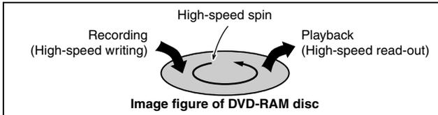
It is called "Live Memory Playback" to start playback of the programme being recorded, with a time-lag between a recording point and a playback point, as shown in the figure below.
