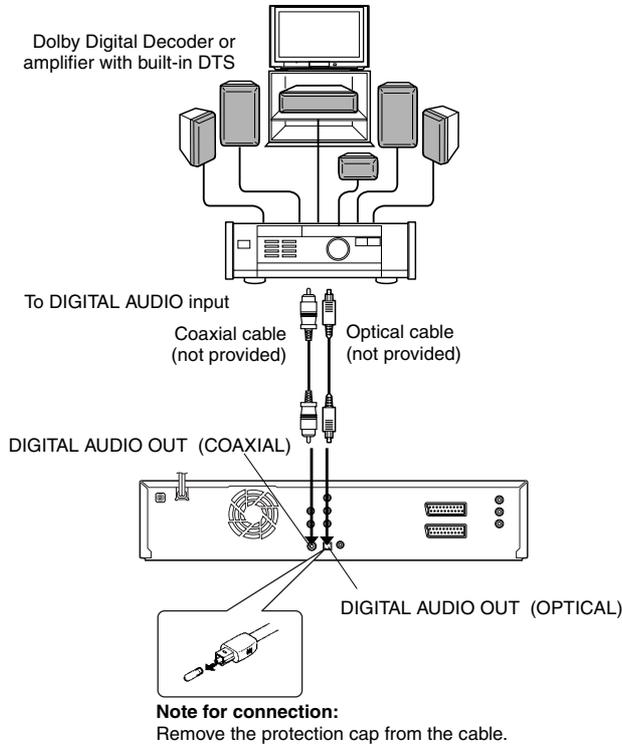
**1** Connect the unit and a Dolby Digital decoder or an amplifier with built-in DTS using either an optional optical cable or an optional coaxial cable.
