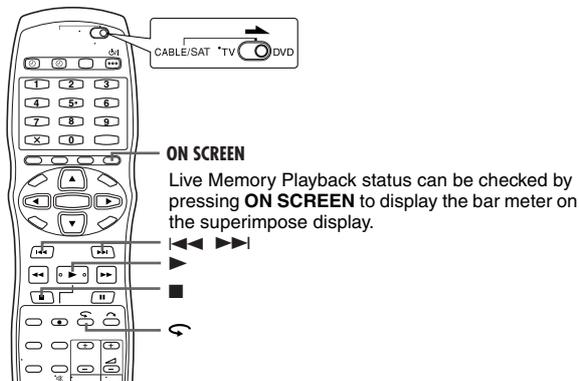
Press **ON SCREEN**. The current status is superimposed on the TV screen.
