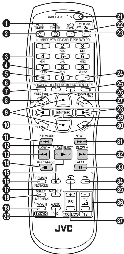
The glow-in-the-dark buttons shown in grey on the illustration above are helpful when using the remote control in darkened rooms.
