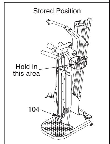
**⚠ WARNING:** Make sure that all of the resistance bars are removed from the “U”-channels before moving the resistance assembly to the stored position.
