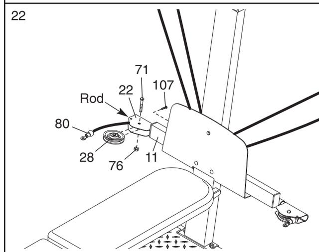
Insert the Swivel Arm (22) into the welded tube on the Cross Tube (11). Secure the Swivel Arm with an M4 x 5mm Screw (107).
