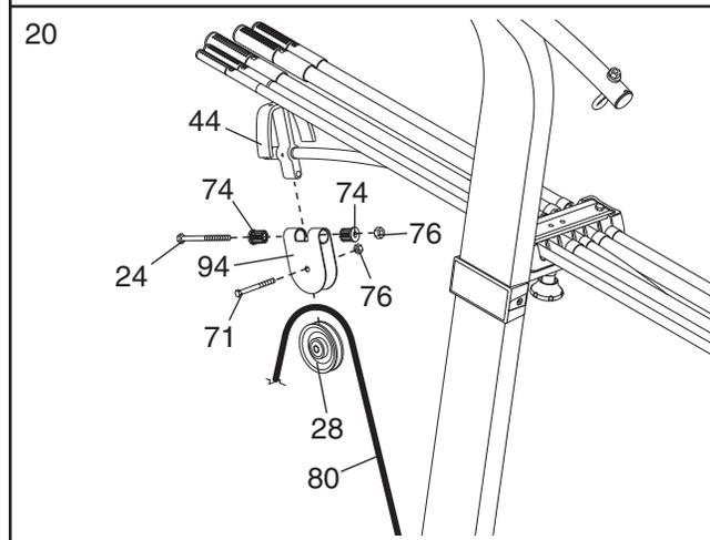
Wrap the Long Cable (80) around a 90mm Pulley (28). Attach the Pulley inside of the Pulley Housing (94) with an M10 x 42mm Button Head Bolt (71) and an M10 Nylon Locknut (76).
