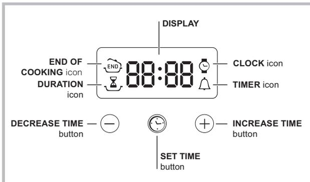
! The Main Oven (only) can be controlled by the automatic timer.
