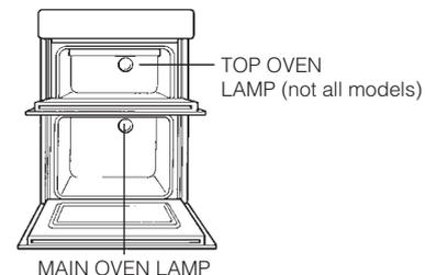
**Warning: To avoid electric shocks - please ensure that the electricity supply to the appliance is switched off and the appliance is fully cold, before cleaning lamp lens.**
