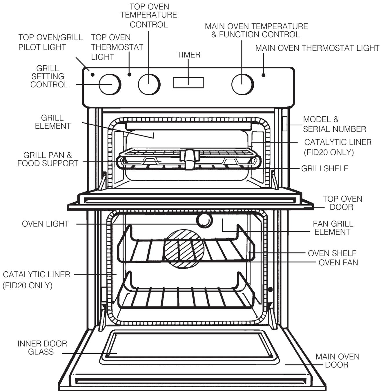
**NEVER** line the shelves, floor or sides of the oven or grill with aluminium foil as overheating and damage may result.
