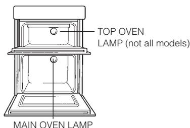
**Warning: To avoid electric shocks - please ensure that the electricity supply to the appliance is switched off and the appliance is fully cold, before removing the lamp lens.**
