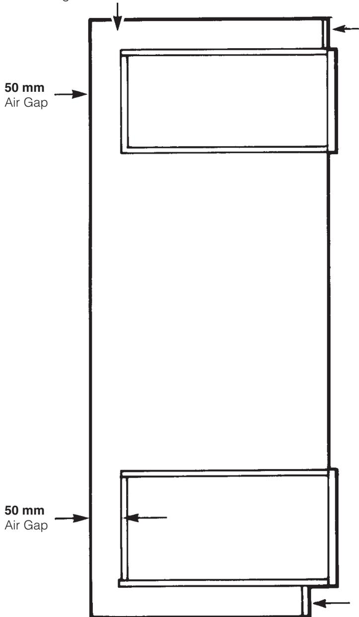
Ventilation Slot required here if the cabinet does not fit to the ceiling - 51mm x 457mm min. area
