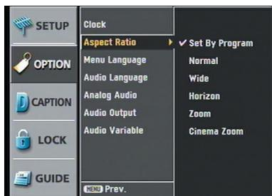
Options to view a picture with a normal (4:3) aspect ratio at 720p or 1080i mode output format.
