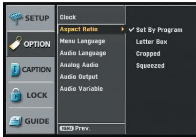
Options to view a picture with a wide (16:9) aspect ratio at 480i or 480p mode output format.
