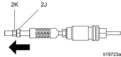
3. Tighten the nuts together to fix them in the new position.
