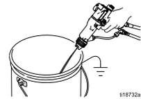
6. Shut off or disconnect the solvent line.
