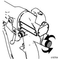
15. Fully open the atomizing air restrictor valve (G) clockwise.
