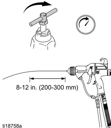
21. Turn on the air to the gun. Turn ON (I) the ES On-Off switch (J).
