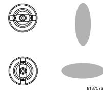
13. Fully open the fan air adjustment valve (F) counterclockwise.
