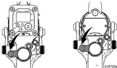
17. Set the gun air regulator to deliver a minimum 45 psi (0.32 MPa, 3.2 bar) at the gun when triggered, to ensure full spraying voltage. See the table below.
