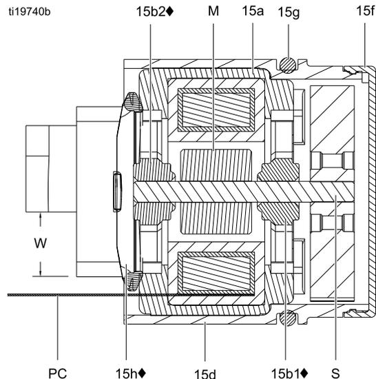
Figure 29 Alternator Cross-Section
