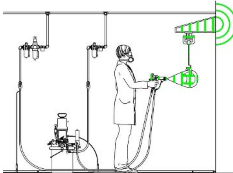
Figure 13 Ground the Object Being Sprayed
