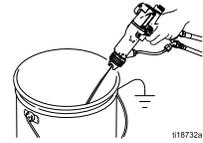
3. Change the fluid source to solvent, or disconnect the fluid line and connect a solvent supply line to the gun.
