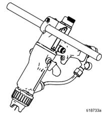
8. When ready to spray again, reconnect the fluid supply line. Follow the [Gun Setup Checklist, page 18](#).
