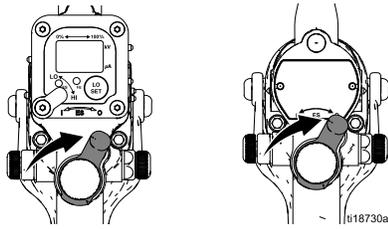
20. Start the pump. Adjust the fluid regulator until the stream from the gun travels 8-12 in. (200-300 mm) before falling off. Typically, if fluid pressure is below 5 psi (.04 MPa, 0.4 bar) or above 30 psi (0.21 MPa, 2.1 bar), a change of nozzle size is recommended.
