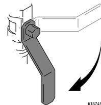
5. If the nozzle or hose is completely clogged or pressure is not fully relieved, slowly loosen the hose end coupling. Now clear the nozzle or hose.
