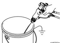
4. Open the pump drain valve, having a waste container ready to catch the drainage. Leave the pump drain valve open until you are ready to spray again.
