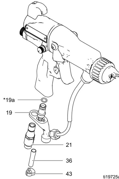
Figure 40 Air Inlet Fitting and Air Exhaust Valve
