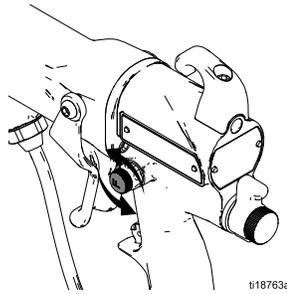
14. Fully open the fluid adjustment valve (H) counterclockwise.
