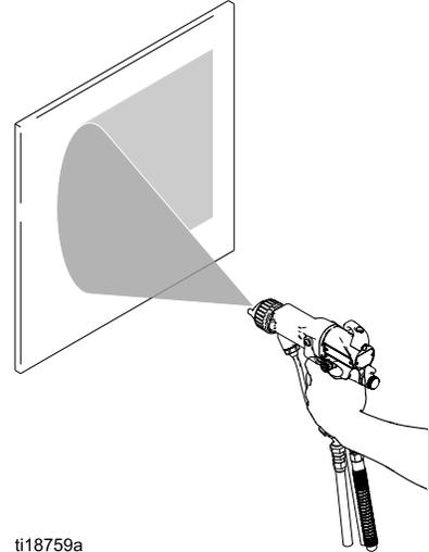
23. Adjust the fan air adjustment valve: clockwise for a narrower pattern, counterclockwise for a wider pattern.
