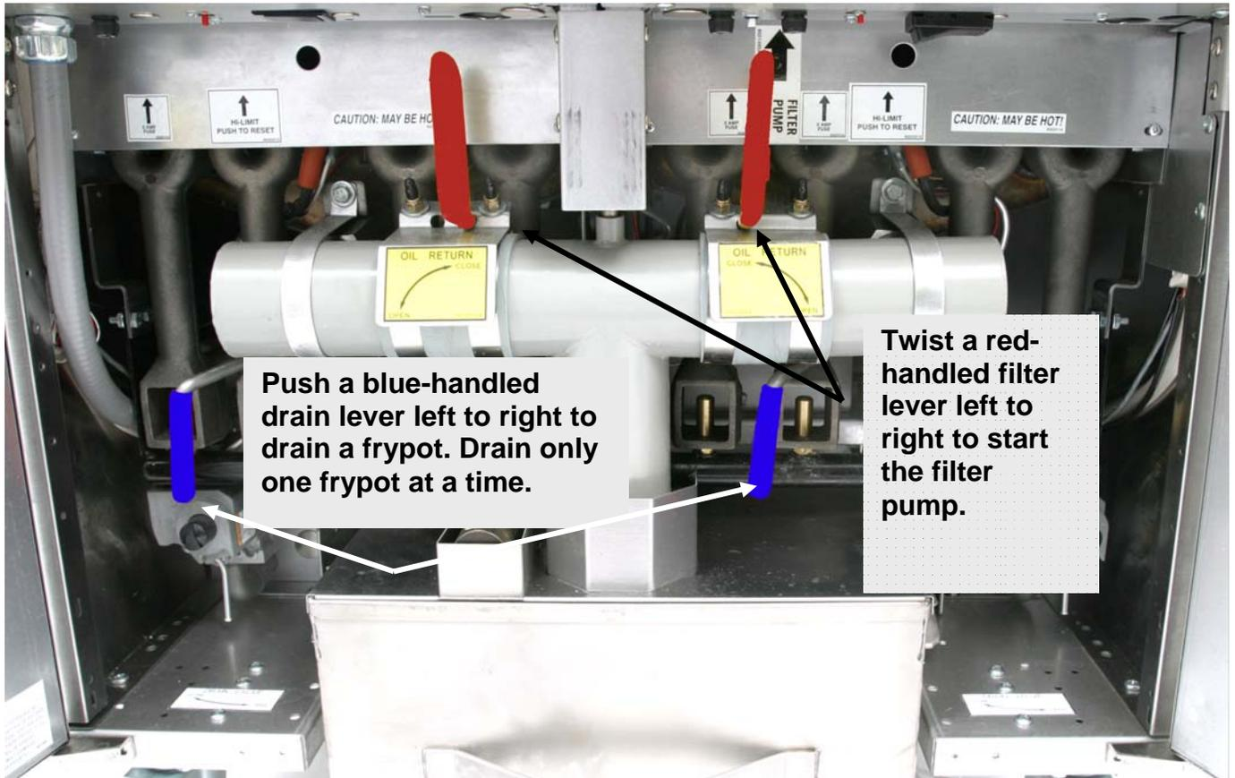
4. After ensuring the filter pan is correctly positioned under the drain tube and the pan are properly connected, drain the frypot into the filter pan. Drain only one frypot at a time.
