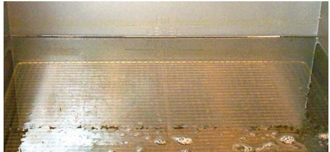
Add oil until the oil level is at the top OIL LEVEL line. DO NOT OVERFILL THE FRYPOT.
