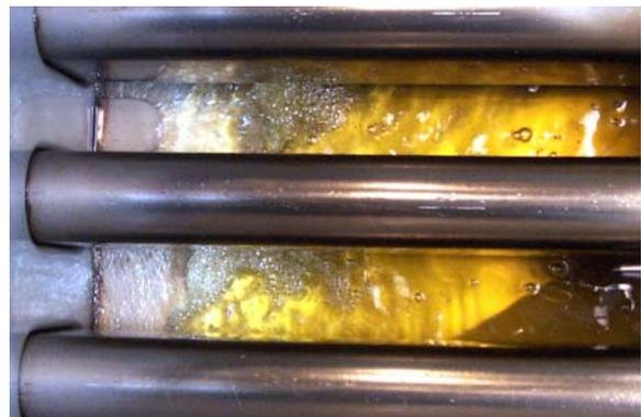
Polishing the oil removes suspended particles, which increases the life of the oil.
