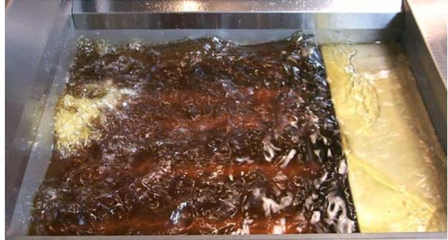
Allow the oil to bubble for 10-15 seconds to ensure evacuation of all shortening/oil in the return lines.
