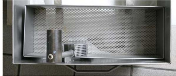
Empty the filter pan crumb tray into a fire-proof container at the end of frying operations each day. **DO NOT ALLOW CRUMBS TO ACCUMULATE IN TRAY.**
