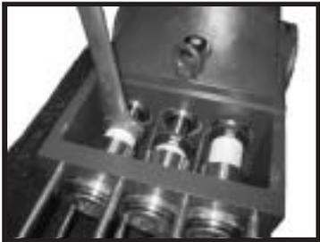
4. Separate plunger connection (36A) from crosshead (25) by means of two open-end wrenches (size 22 and 27). Pull seal sleeves (39) out of their fittings in the crankcase.
