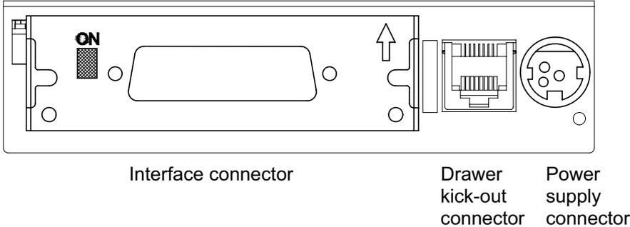
※ When the Dip Switch is “ON” on the Serial Interface Board, DTR and RTS are connected each other.
